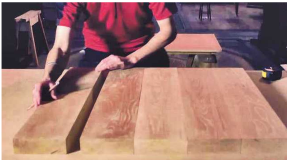
▲ Pic.3 Once cut, the planks are laid out and the grain matched as best as possible
